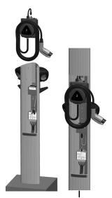
**NOTE:** On the CT2025, insert the cable assembly into the main body's access panel opening, then slide down.
