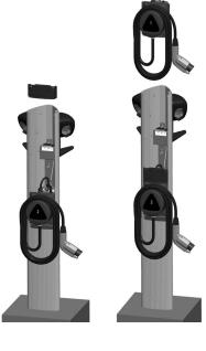
**NOTE:** On the CT2025, insert the filler panel and cable assembly into the main body's access panel opening, then slide down
